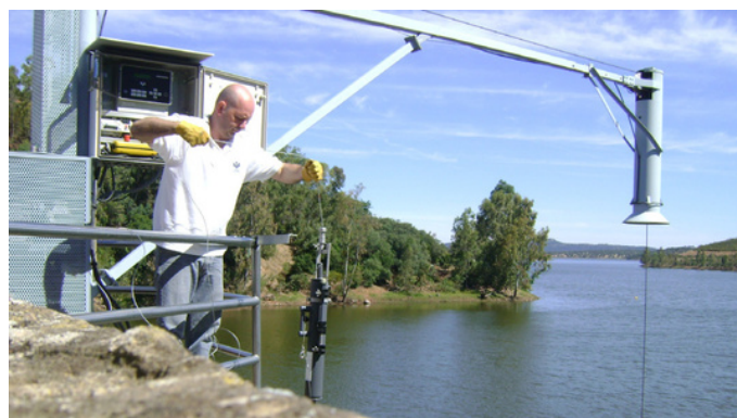
Figure 5. Automatic system for measuring the quality of reservoir water at different depths. Technician checking values.
