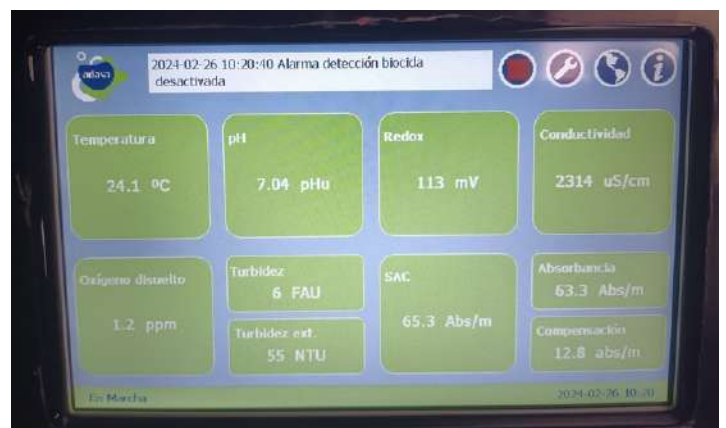
aquaTest-MO measures different microbiological and physico-chemical parameters.
