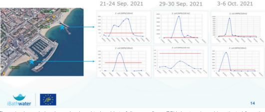
The episode mode has been developed to be able to follow up after a DSU due to rain and is activated from the control center. The equipment switches from daily mode to continuous measurement until the value at which the water quality has recovered, allowing to know the moment when the quality is optimal again.
