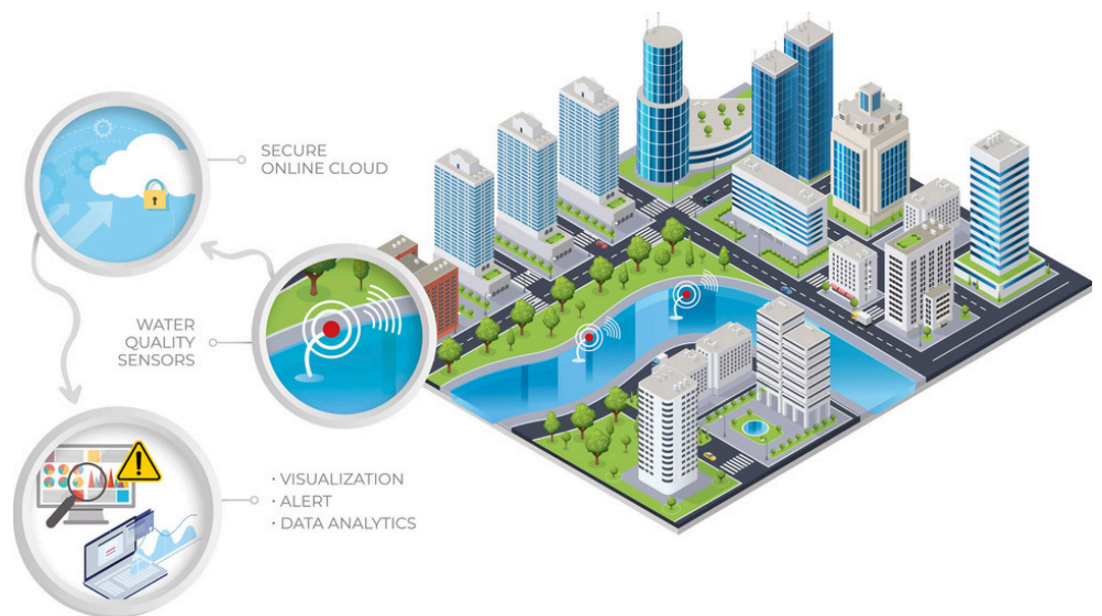
Adasa developed an on-line water quality monitoring system for Singapore's urban drainage systems.
